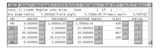
The array data is entered using SPECIAL>>Surface Control>>Regular Lens Array. Since there is a single row of lenses, the *x* spacing is 0. The number of lenses is controlled by the aperture of the channel surface (surface 1). Only the vertex of each channel needs to be within the aperture of the channel surface to be included in the array, although here the aperture has been set to enclose the entire array surface.
