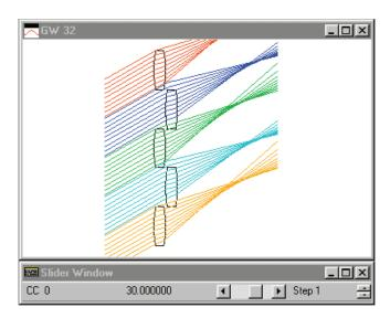
When the setup window is closed, the slider-wheel window appears, and you can see that at wide angles, rays do not follow their actual trajectories, because of the way that channels are selected. This is not a problem for narrow fields or when surfaces are not displaced from the channel surface, as you can verify by manipulating the slider.
