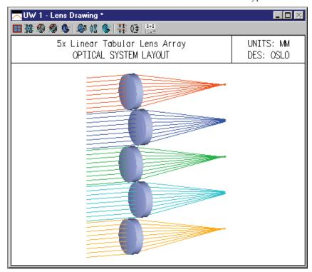
The main surface data spreadsheet is identical to the one for the regular array. The difference is in the array data spreadsheet (SPECIAL>>Surface Control>>Tabular Lens Array), which enumerates the coordinates of the vertices of each element (channel) in the array. Note that a z displacement has been added to elements 2 and 3. This is not accounted for in the above drawing, which shows rays traced to the nominal image surface, from a field point 10 degrees off axis.
